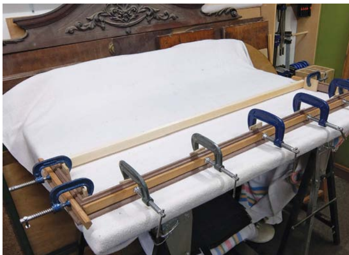
The cove moulding glued and clamped to the cornice frame
